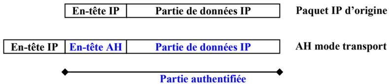
**Figure 6.7.** Encapsulation AH en mode transport
